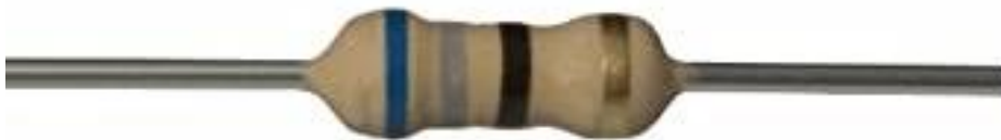
Figure 7. 68 Ohm resistor – the coloring coding
