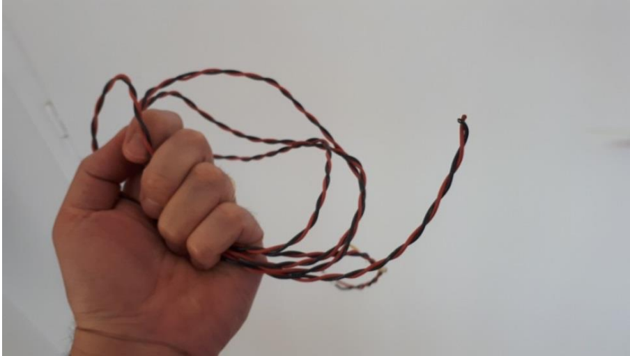
Figure 2. Regular wires twisted to form the control signal line
