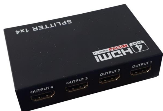
Figure 4.14 Example HDMI Splitter – Outputs
