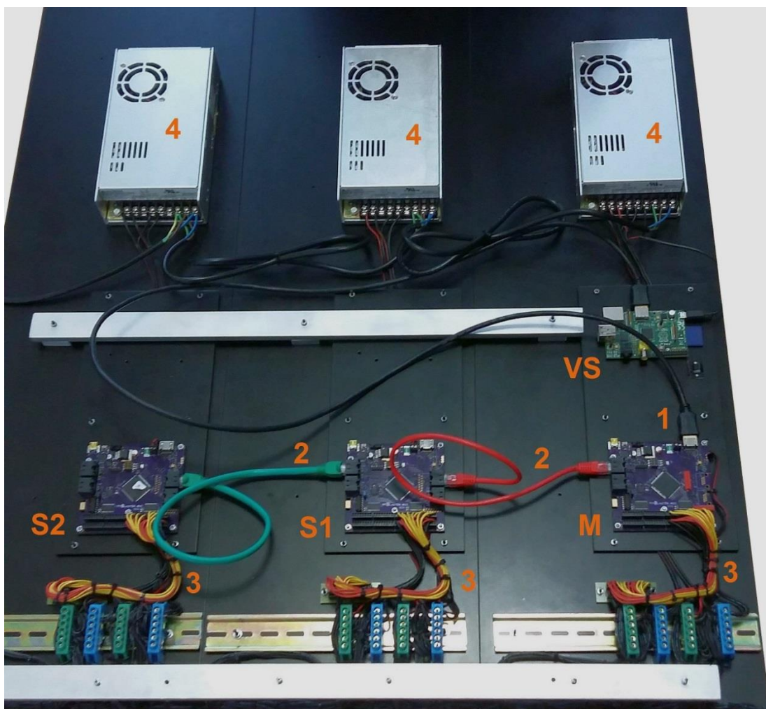
Figure 5.7 Demo Display Structure in the Multi-Controller Topology
