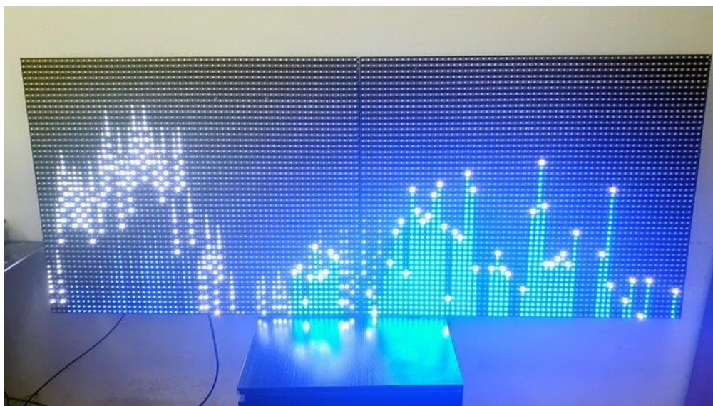
Figure 1.5 Pixblasters Demo Made Using LED Strips Glued to Aluminum Plates
