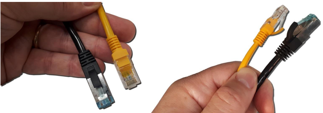
Figure 8.5 The STP (black) and the UTP (yellow) Cables
